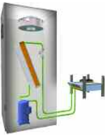
A - Air-cooled with remote condenser
